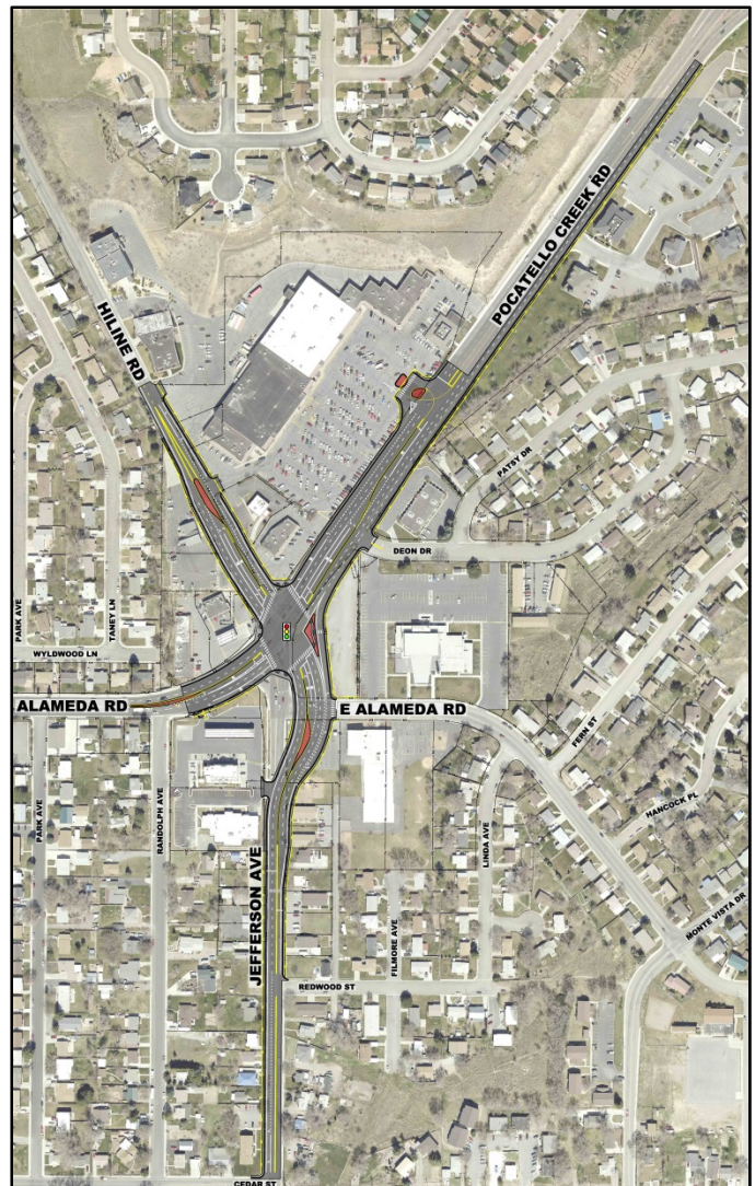
Figure 10. Alternative 14A – Conventional intersection with free northbound right-turn movement – see Appendix A for larger display
